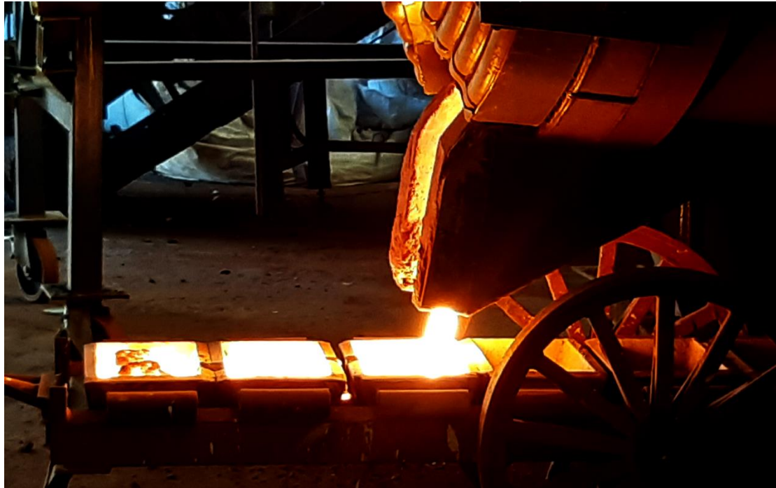
Figure 4. BR pig iron production at MYTILINEOS Pyro-Pilot Plant.
