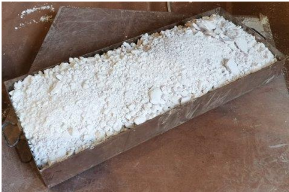
Figure 6. Bayerite precipitate from BR processing at MYTILINEOS.
